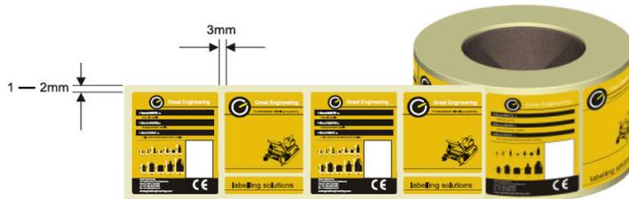
Some customers may choose to build the label gap into their labels as the alternate on the roll, as shown below:
